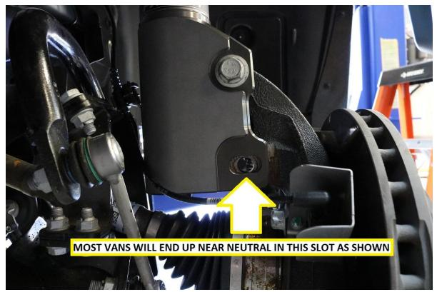
25) With the lower strut bolt installed, snug both upper and lower strut bolts. Use a 18mm wrench for the bolt head. 21mm wrench for the nut.
