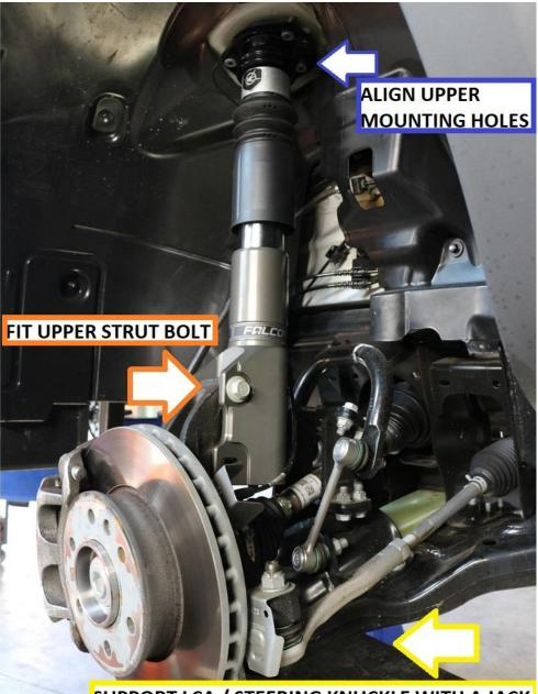
SUPPORT LCA / STEERING KNUCKLE WITH A JACK
