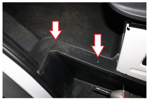
3) The passenger side upper strut bolts can be accessed by pulling up the tool kit cover panel in the passenger footwell. Use a large flat blade screwdriver to rotate the lock knobs on the kick panel so they are horizontal.
