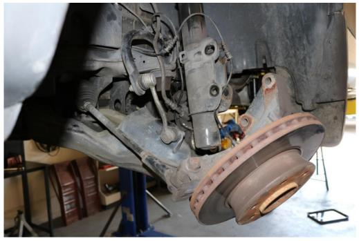
12) Fully remove the strut by removing the four upper strut bolts inside the cabin of the vehicle. Use a 13mm socket / wrench for removal.
