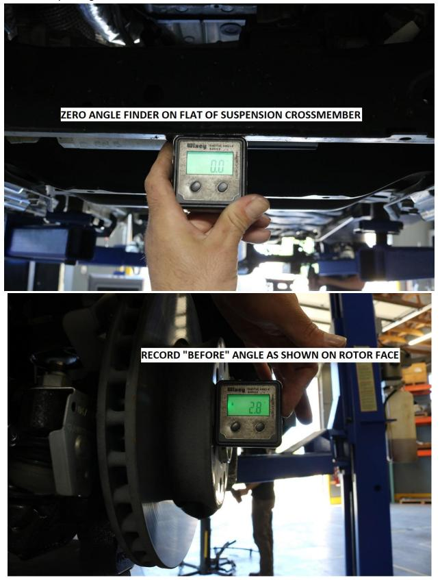
10) With the "before" camber measurements recorded, support / raise the lower control arm about 3/8" (10mm) to remove tension from the strut. Use a 21mm socket to remove the 2 bolts securing the strut to the steering knuckle.
